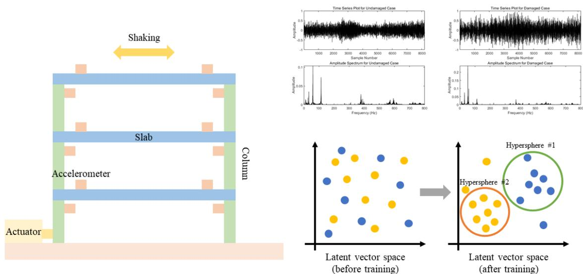
Fig. 1 Shake table test and support vector data description
